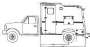
TARP WIRELINE UNIT
